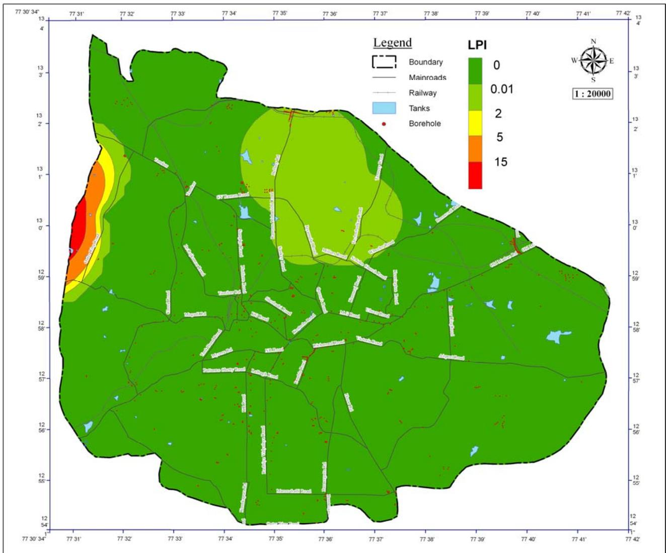
**Fig. 4: Liquefaction potential hazard map**
