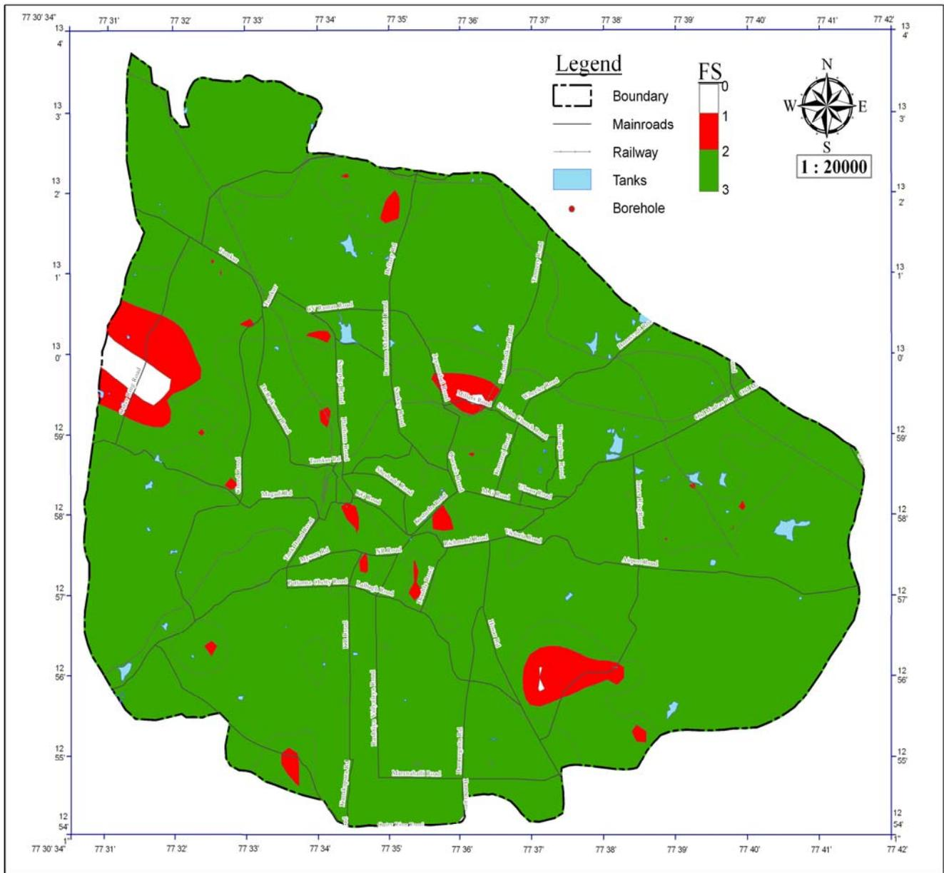
Fig. 2: Map of factor of safety against liquefaction
